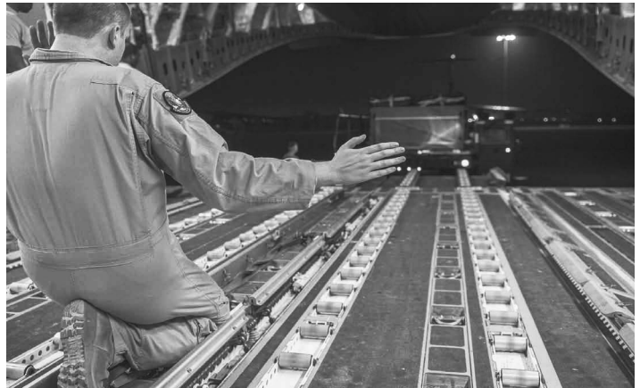
Airlift delivers critical supplies - 1/22/2013 - U.S. Air Force Tech. Sgt. Russell Johnson, 816th Expeditionary Airlift Squadron loadmaster, guides a 10 K-Loader to the cargo area of a C-17 Globemaster III at a deployed location in Southwest Asia, Jan. 10. The loadmaster performs the calculations and plans cargo and passenger placement to keep the aircraft within permissible center of gravity limits throughout the flight. Johnson is deployed from the 14th Airlift Squadron at Joint Base Charleston, S.C. (U.S. Air Force photo/ Tech. Sgt. Dennis J. Henry Jr.)
